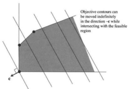
Figure 1.7. Unbounded optimal objective value.
